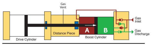
The pistons below are traveling to the left and compressing the gas in chamber "A" while pulling gas into chamber "B".
