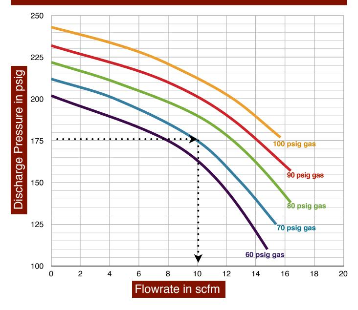
Use the curves above to determine the Model 43AAV34 gas pressure booster maximum discharge flowrate for a given set of operating conditions. In the example shown above, a maximum discharge pressure of 175 psig is desired. The drive air pressure is 80 psig for all points on the curves. The gas supply pressure is 70 psig. Follow the 175 psig line until
