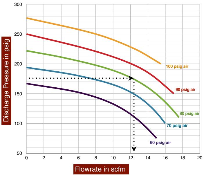
Use the curves above to determine the Model 43AAV34 gas pressure booster maximum discharge flowrate for a given set of operating conditions. In the example shown above, a maximum discharge pressure of 175 psig is desired and 80 psig supply air is available. Follow the 175 psig line until it intersects with the
