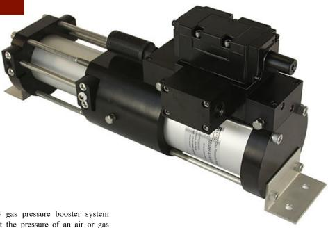
The Model 43AAV34 gas pressure booster system uses shop air to boost the pressure of an air or gas stream. The drive air piston reciprocates automatically and drives the gas compressor piston. The booster is non-lubricated and uses filled Teflon® piston seals and rod seals. It requires no electricity, cooling water, or air-line lubricator and is explosionproof.
