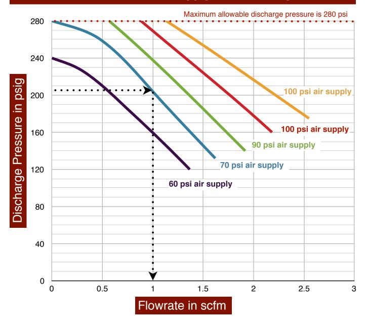
Use the curves above to determine the Model RL403S air pressure booster maximum discharge flow rate for a given set of operating conditions. In the example shown above, a discharge pressure of 205 psig is desired and 70 psig supply air is available. Follow the 205 psig line until it intersects with the 70 psig supply
