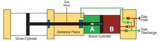
The distance piece is designed to ensure that the gas in the boost cylinder is isolated from the air in the drive cylinder. There are piston rod seals at each end of the distance piece, and the distance between the rod seals is greater than the stroke length of the booster. Consequently, the section of piston rod which penetrates the drive cylinder never penetrates the boost cylinder and vice versa.
