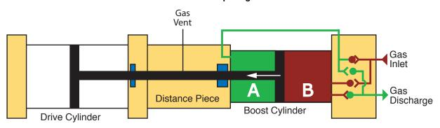
The distance piece is designed to ensure that the air in the boost cylinder is isolated from the air in the drive cylinder. There are piston rod seals at each end of the distance piece, and the distance between the rod seals is greater than the stroke length of the booster. Consequently, the section of piston rod which penetrates the drive cylinder never penetrates the boost cylinder and vice versa.
