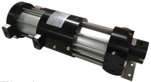
The Model 420TAAV090 air/gas pressure booster system uses shop air to boost the pressure of an air or gas stream. The drive air piston reciprocates automatically and drives the gas compressor piston. The booster is non-lubricated and uses filled Teflon® piston seals and rod seals. It requires no electricity, cooling water, or air-line lubricator and is explosion proof.
