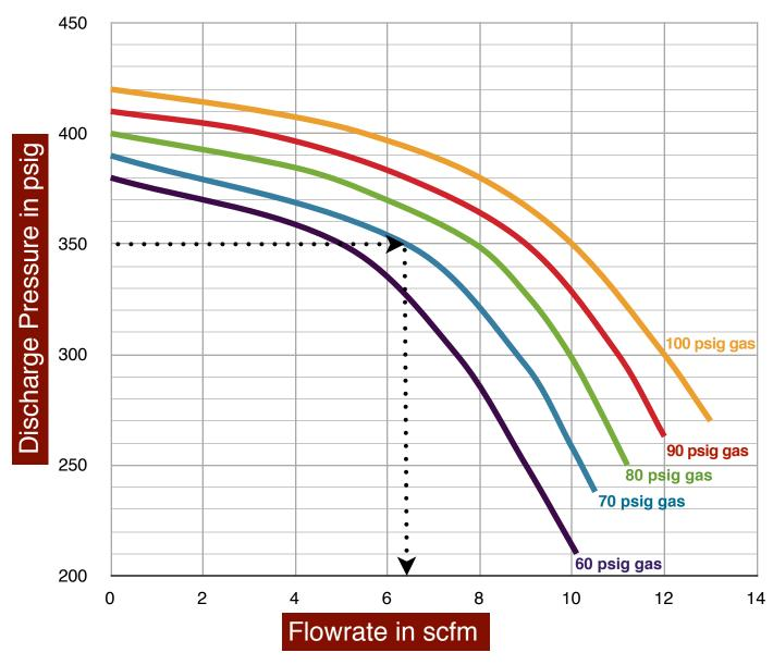
Use the curves above to determine the Model S42N5 gas pressure booster maximum discharge flowrate for a given set of operating conditions. In the example shown above, a maximum discharge pressure of 350 psig is desired. Note that the drive air pressure is 80 psig for all points on the curves. For a gas supply pressure of 70 psig, follow the
