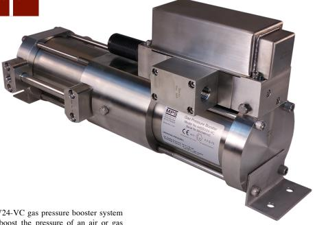
The Model 44SSV24-VC gas pressure booster system uses shop air to boost the pressure of an air or gas stream. The drive air piston reciprocates automatically and drives the gas compressor piston. The booster is non-lubricated and uses filled Teflon® piston seals and rod seals. It requires no electricity, cooling water, or air-line lubricator and is explosionproof.
