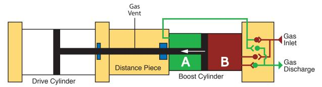
The distance piece is designed to ensure that the gas in the boost cylinder is isolated from the air in the drive cylinder. There are piston rod seals at each end of the distance piece, and the distance between the rod seals is greater than the stroke length of the booster. Consequently, the section of piston rod which penetrates the drive cylinder never penetrates the boost cylinder and vice versa.
