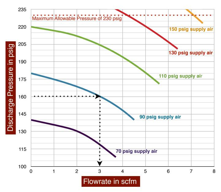
Use the curves above to determine the Model RL12S-D air pressure booster maximum discharge flow rate for a given set of operating conditions. In the example shown above, a maximum discharge pressure of 160 psig is desired and 90 psig supply air is available. Follow the 160 psig line until it intersects with the
