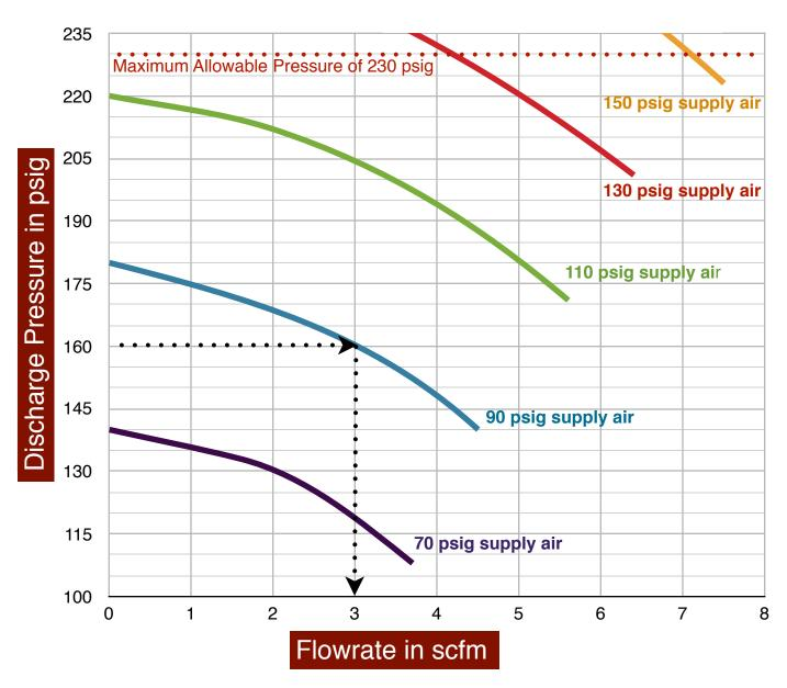
Use the curves above to determine the Model RL12S air pressure booster maximum discharge flow rate for a given set of operating conditions. In the example shown above, a maximum discharge pressure of 160 psig is desired and 90 psig supply air is available. Follow the 160 psig line until it intersects with the
