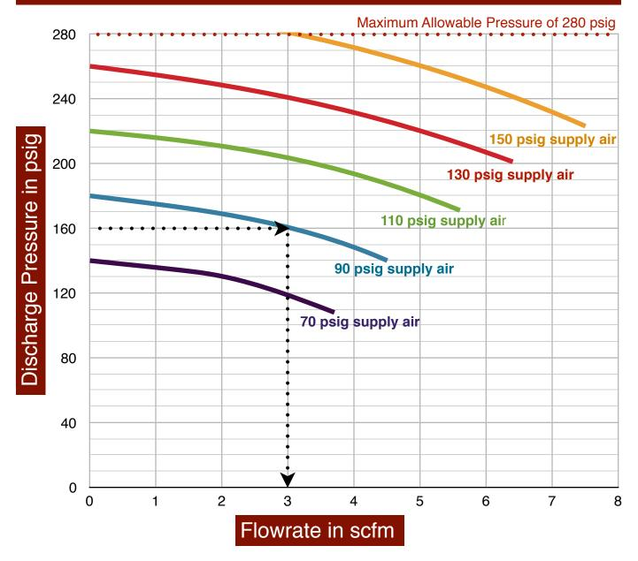
Use the curves above to determine the Model RL03S-D air pressure booster maximum discharge flow rate for a given set of operating conditions. In the example shown above, a maximum discharge pressure of 160 psig is desired and 90 psig supply air is available. Follow the 160 psig line until it intersects with the
