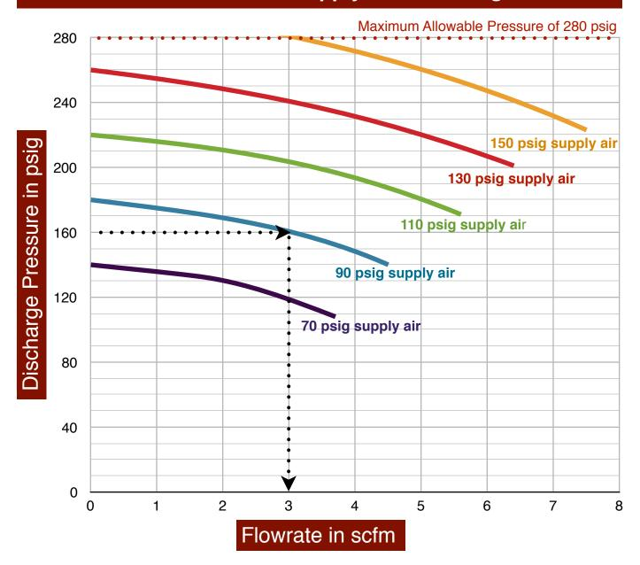
Use the curves above to determine the Model RL03S air pressure booster maximum discharge flow rate for a given set of operating conditions. In the example shown above, a maximum discharge pressure of 160 psig is desired and 90 psig supply air is available. Follow the 160 psig line until it intersects with the
