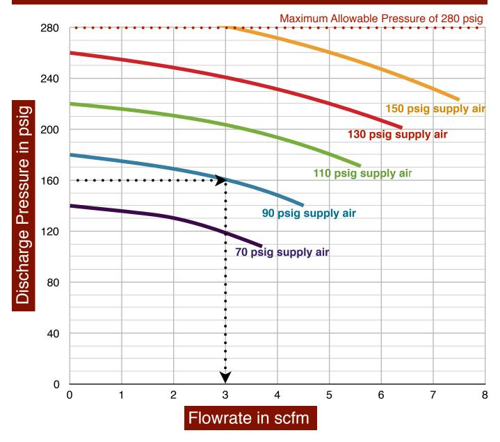
Use the curves above to determine the Model RL00S air pressure booster maximum discharge flowrate for a given set of operating conditions. In the example shown above, a maximum discharge pressure of 160 psig is desired and 90 psig supply air is available. Follow the 160 psig line until it intersects with the
